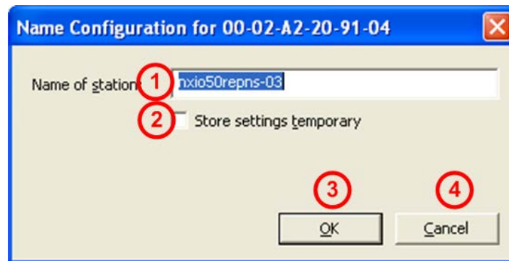
Figure 15: DCP Set Device Name
