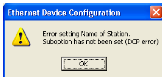
Figure 16: Error when setting Name of Station
